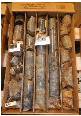
Figure 3 – Photo of oxidized jasperoid breccia from LB21-004, interval 394 - 398 feet (120.1 - 121.3 meters) returned a value of 17.3 g/t Au, surrounding intervals ranged from 8.6 - 12.8 g/t Au. To view image please click here
