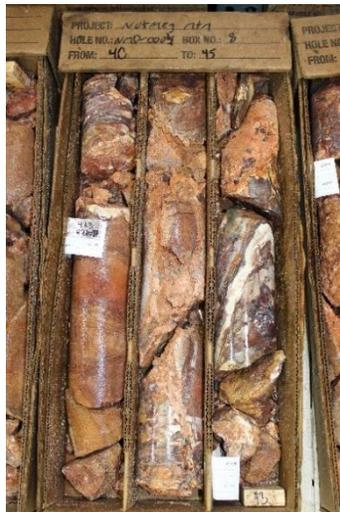
Figure 3 – Core Photos – NMD0004 from 12.2 meters to 13.7 meters (40 to 45 ft.), included in the zone that assayed 11.3 meters of 1.4 g/t Au. [To view image please click here](#)
